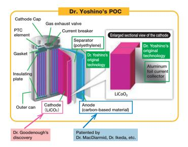
By combining existing technologies with his own, Dr. Yoshino proposed and demonstrated that the lithium ion battery system, in which "charge/discharge is achieved by the traversal of lithium ions through the cathode-anode gap," is capable of delivering the performance necessary for practical application.
