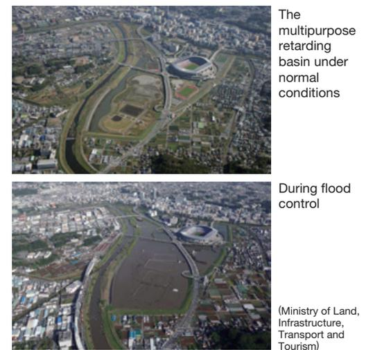
A large-scale multipurpose retarding basin has been created in the Tsurumi River area, which suffered severe damage caused by the Kanogawa Typhoon in 1958. When the river volume increases, the water is channeled into the retarding basin, thereby preventing the flooding of the residential areas.
