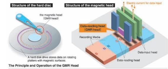
When the GMR head moves, the direction of the magnet of the GMR element is altered by the change in the direction of the magnet on the surface of the disc. As the resistance of the element changes in accordance with GMR effect, it is able to be detected as an electric signal. Thanks to the GMR element, even the slightest change to the magnetic field caused by a minute bit can be detected, and this has resulted in further advancements in the high density of hard discs.
